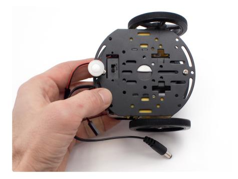
Place the battery box back in between the motors and stick it to the chassis
