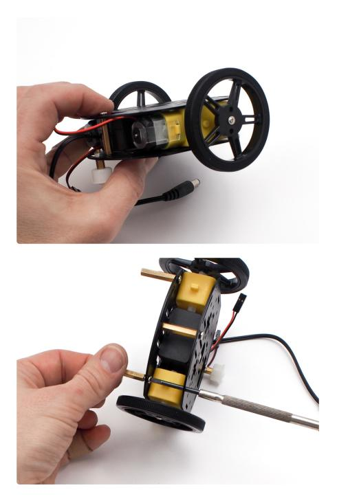
Take a look at the image below and install the brass stand-offs in the same positions. You can insert the stand-off screws through the middle plate and hand tighten the stand-offs while putting a bit of pressure on the screw with your finger. Or, as a tip, you can screw in the stand-off screws with the flat end of the screwdriver, which can reach through the holes in the bottom plate.
