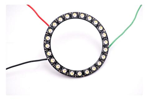
Solder leads to the **DIN**, **+5V**, and **GND** pins on the NeoPixel ring. Solid core hookup wire is a nice choice, as it can serve double duty as the structural connection to hold the ring in place underneath.
