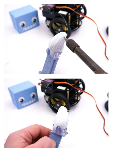
Use a couple of pieces of double stick foam tape to mount the micro servo and candy dispenser to the top plate of CurieBot. You can also drill a small hole into the foot of the candy dispenser base and screw it in place on one of the robot's brass standoffs.
