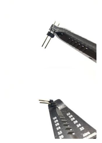
For this next step, you will need a set of pliers. First, grab the long header pins that are attached together and break them into 2 sets of 2 header pins. Then, grab them in the pliers like shown here, and then slightly bend them so they look like the next picture.
