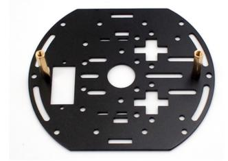
Attach two of the brass standoffs onto the black chassis layer.
