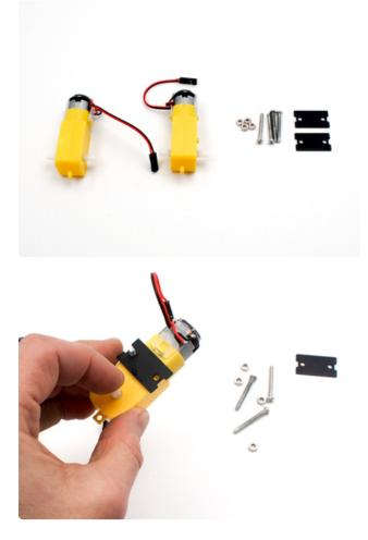
To start, take the two motors, four long screws, four nuts, and two black panels.
