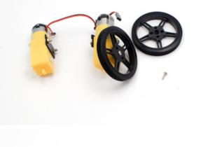
Fit the wheels onto the white knob on the motors, they will snap nicely onto the oval center.
