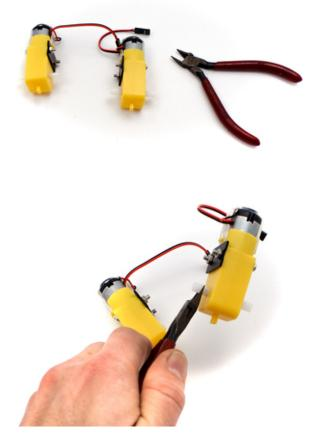
To make space for the 9V battery pack later, trim the excess off of the inner motor wheel shaft on each motor. Grab some diagonal cutters (scissors or a hobby knife will work in a pinch) and trim off about half the length of the motor wheel shaft that is on the same side as the black plate you affixed.
