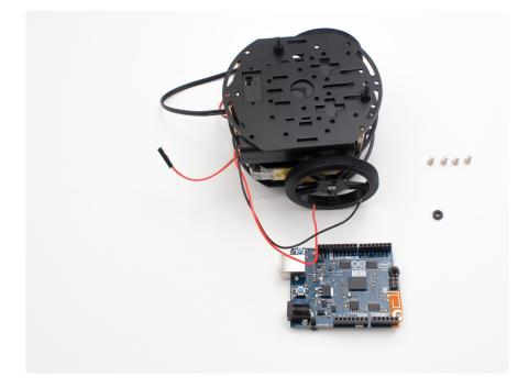
Screw the four brass standoffs into place with the small metal screws.
