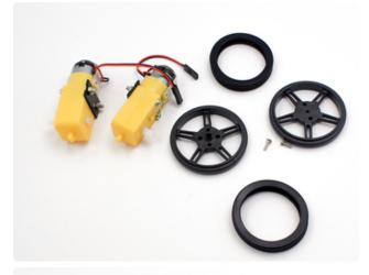
Take the two wheels, rubber treads, and 2x small screws found in the same bag as the wheels.
