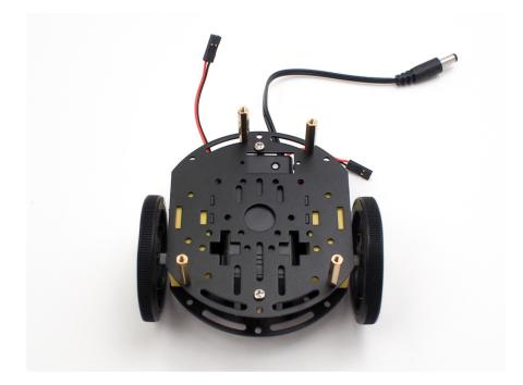
Once you have the stand-offs in place as shown in the image above, let's place the battery box in the correct spot as shown in the image below.
