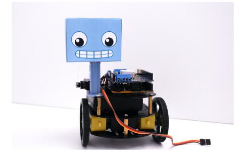
Plug the servo cable into the Servo 1 port on the MotorShield.
