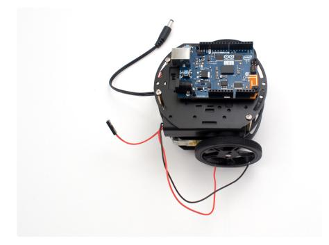
Route the wires up through the chassis layers for connecting them later to the MotorShield.
