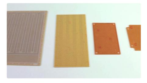
There are many different types available, but at the most basic level, perfboard is a perforated board - providing a grid of holes usually surrounded by metal "pads" which you can securely solder components to.
