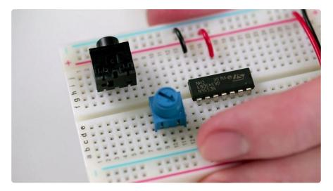
You can find a lot of components that are "breadboard friendly", meaning that their lead-spacing matches up nicely with a breadboard, so they pop right into place.
