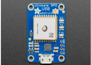
The USB version doesn't have those GPIO pins broken out. Instead it has a single USB serial port. There's 4 pads to the right side that are the USB pinouts for when you want to solder it directly to a USB host controller.
