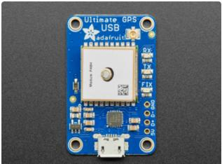
You can also skip the USB console cable, and just plug a USB C or Micro B cable directly from your computer to the Ultimate GPS USB
