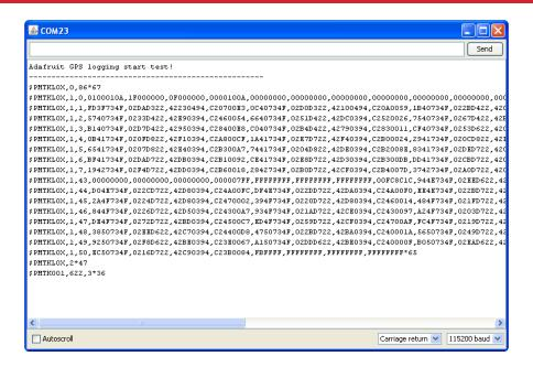
Copy and paste all the text after the —-'s (starting with \$PMTKLOX,0,86\*67 and ending with \$PMTK001,622,3\*36) then paste it into the box located on this page (https://adafru.it/cFg)
