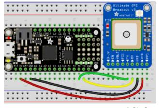
If you're using a board with hardware serial support, like this Feather M0, wire up VIN to 3.3V (since that is the logic level of the Feather M0), GND to ground, and GPS RX to Feather TX and GPS TX to Feather RX.
