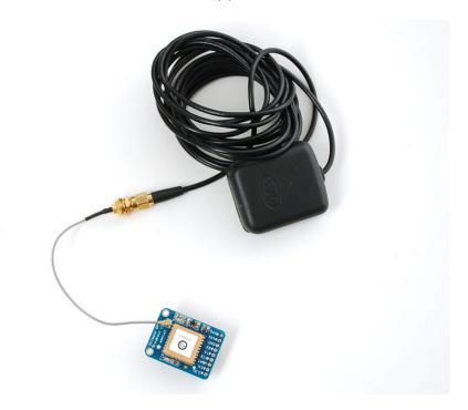
All Ultimate GPS modules have a built in patch antenna - this antenna provides -165 dBm sensitivity and is perfect for many projects. However, if you want to place your project in a box, it might not be possible to have the antenna pointing up, or it might be in a metal shield, or you may need more sensitivity. In these cases, you may want to use an external active antenna. (http://adafru.it/960)
