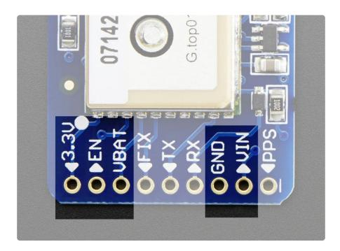
These are the pins that are involved with powering the GPS. Starting from the right are the **required** power pins:
