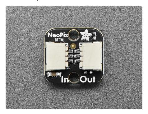
The two mounting holes are M2 size and have clearance for the screw head, or could be used for sewing onto a fabric backing or attaching to a small model. Of course this design will never be as affordable as a pre-made strand with dozens of LEDs, but
