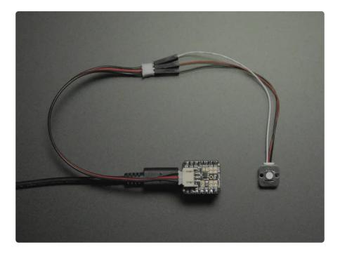
This little breakout makes it easy to add a single NeoPixel to a project, with mounting holes and a pluggable connector. The PCB is less than 0.5"x0.5" and comes with two 3-pin JST SH 1mm pitch connectors (http://adafru.it/5755) for input and output. On the opposite side, a 5050 (5mm square) classic RGB NeoPixel that can be powered and controlled with 3.3V or 5V power.
