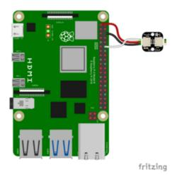
Pi 3V to NeoPixel JST SH VIN (red wire) Pi GND to NeoPixel JST SH GND (black wire)
