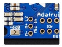
We break out the microphone/line in inputs, for recording audio. Some basic analog filtering is required depending on the electret microphone or amplifier. Check the VS1053 datasheet for how to connect up a mic!
