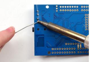
Solder the four pins with plenty of solder
