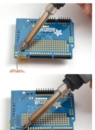
Then flip the board over and solder the 6 pins
