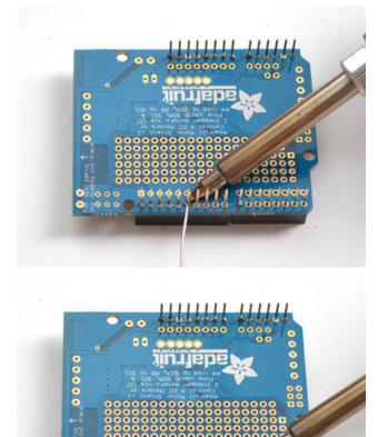
Once you've tacked and straightened all the headers, go back and solder the remaining pins for each header.
