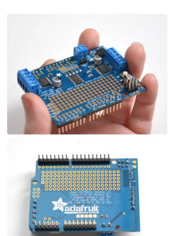
Finally, break off a 2-pin piece of header and place it next to the POWER terminal block, short legs down, tape it in place if necessary and solder it in.
