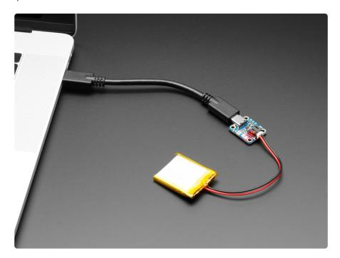
Charging is performed in three stages: first a preconditioning charge, then a constant-current fast charge and finally a constant-voltage trickle charge to keep the battery topped-up. The charge current is 100mA by default, so it will work with any size battery and USB port. If you want you can easily change it over to 500mA mode by soldering closed the jumper on the front, for when you'll only be charging batteries with 500mAh size or larger.
