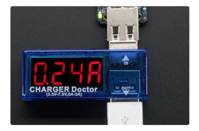
If you want to check the exact current draw during charge, try out a Charger Doctor between the USB port and charger. (http://adafru.it/1852)
