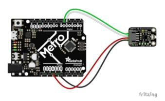
Board 5V to VIN (red wire) Board GND to GND (black wire) Board pin 5 to IRin (white wire) Board pin 6 to IRout (green wire)
