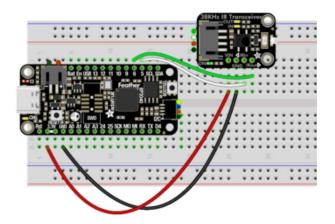
Board 3V to VIN (red wire) Board GND to GND (black wire) Board pin 5 to IRin (white wire) Board pin 6 to IRout (green wire)
