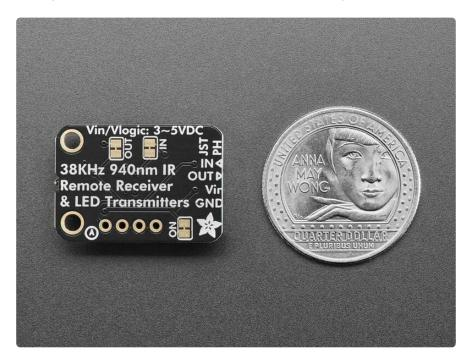
For the emitter half, we use the <u>same schematic and setup as our "High Power IR LED</u> <u>Emitter" breakout (http://adafru.it/5639)</u>, with an onboard N-Channel FET driver, to blast 100mA-200mA of current pulsing through each LED for 10+ meters of range!
