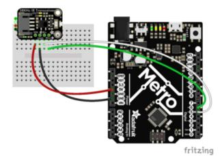
Board 5V to VIN (red wire) Board GND to GND (black wire) Board pin 5 to IRin (white wire) Board pin 6 to IRout (green wire)
