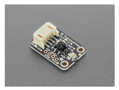
Each STEMMA board is a fully assembled and tested PCB, but no cable. No soldering is required to use it, but you will need to pick up <u>a 2mm pitch, 4-pin STEMMA JST PH</u> <u>cable (https://adafru.it/1a3Y)</u>. Alternatively, if you do want to solder, there's a 0.1" spaced header for power/ground/signals.
