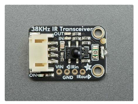
**Please Note:** to make this board easy to use, we have both solder-able breakout pads and also a JST PH 4-pin cable. We often use JST PH cables for I2C but this board **does not use I2C** - the green wire is data from a microcontroller to be emitted over the IR LED, the white wire is demodulated IR remote signal data to a microcontroller. The black wire is ground, red wire is 3V~5V power and logic level.
