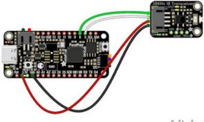
Board 3V to VIN (red wire) Board GND to GND (black wire) Board pin 5 to IRin (white wire) Board pin 6 to IRout (green wire)
