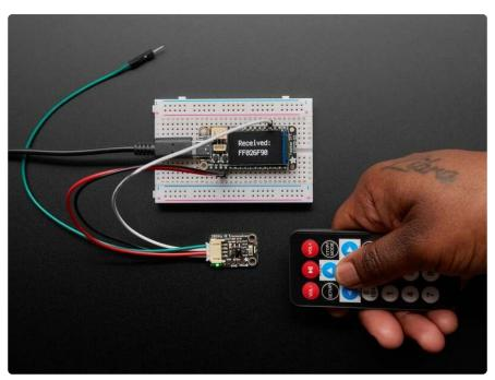
We've got a <u>high-powered infrared emitter board</u> (http://adafru.it/5639), and a <u>super-</u> <u>sensitive infrared remote receiver board</u> (http://adafru.it/5939) - but why buy two boards when you can pick up one that does both? This board is the **Adafruit Infrared Tranceiver breakout**, which can transmit and receiver 940nm remote control data in one handy solder-free package.
