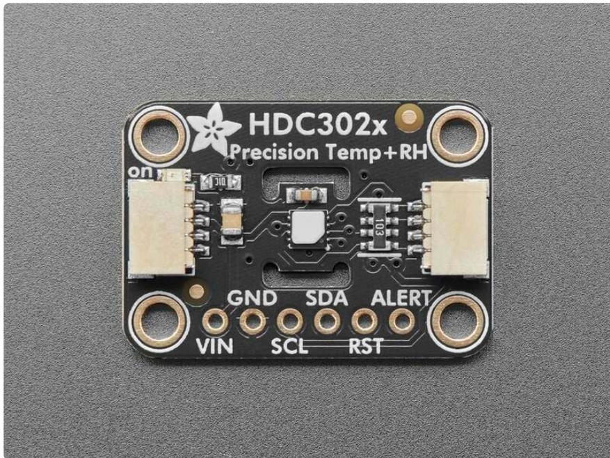
Adafruit stocks a large number of Temperature/Humidity sensors, so you're probably wondering why another one? Well, this **Adafruit HDC3021 Precision Temperature & Humidity Sensor** breakout features the highest accuracy & precision one we've see so far!
