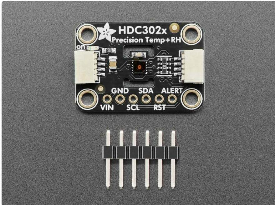
Such a lovely chip - so we spun up a breakout board with the HDC3021 and some supporting circuitry such as pullup resistors and capacitors. To make things even easier, we've included [SparkFun Qwiic \(https://adafru.it/Fpw\)](https://adafru.it/Fpw) compatible [STEMMA QT \(https://adafru.it/Ft4\)](https://adafru.it/Ft4) connectors for the I2C bus so you don't even need to solder! [QT Cable is not included, but we have a variety in the shop \(https://adafru.it/17VE\)](https://adafru.it/17VE).
