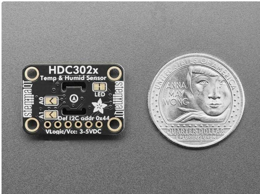
This sensor has a true I2C interface for easy interfacing with only two wires (plus power and ground!). That makes it preferable to the janky DHT11/DHT22 sensors.
