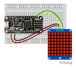
Microcontroller 3V to LED Matrix VIN Microcontroller GND to LED Matrix GND Microcontroller SCL to LED Matrix SCL Microcontroller SDA to LED Matrix SDA
