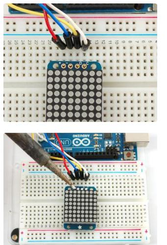
Place the soldered backpack on top of the header.
