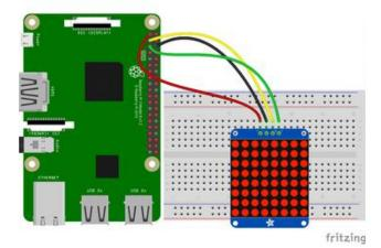
Raspberry Pi 3.3V to LED Matrix VIN Raspberry Pi GND to LED Matrix GND Raspberry Pi SCL to LED Matrix SCL Raspberry Pi SDA to LED Matrix SDA
