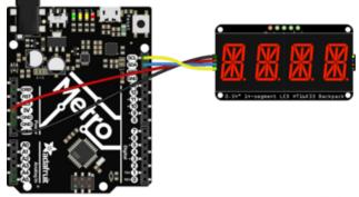
Board 5V to backpack Vio (red wire) Board GND to backpack GND (black wire) Board SCL to backpack SCL (yellow wire) Board SDA to backpack SDA (blue wire)
