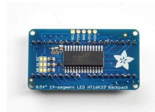
Check your work, making sure each pin is nicely soldered, and there's no cold solder joints or shorted pins
