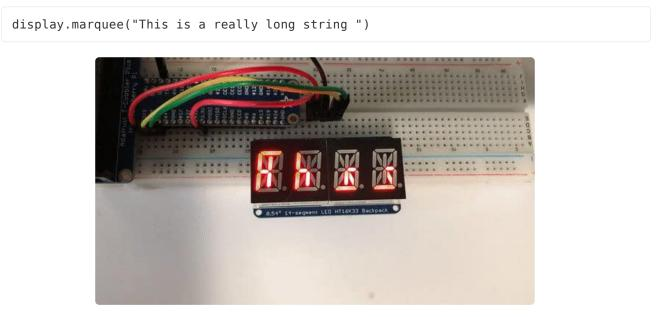
By default it is 0.25 seconds, but you can change this by providing a second parameter. You can optionally pass **False** for a third parameter if you would not like to have it loop. So if you wanted each character to display for half a second and didn't want it to loop, you would use the following:
