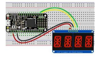
Microcontroller 3V to AlphaNumeric Display I2C VIN Microcontroller 3V to AlphaNumeric Display VIN Microcontroller GND to AlphaNumeric Display GND Microcontroller SCL to AlphaNumeric Display SCL Microcontroller SDA to AlphaNumeric Display SDA
