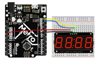
Backpack + (VCC) to microcontroller 5V (if using a board with 5V logic, otherwise use 3V for boards with 3V logic) (red wire) Backpack - (GND) to microcontroller GND (black wire) Backpack D (SDA) to microcontroller SDA (blue wire) Backpack C (SCL) to microcontroller SCL (yellow wire) To assemble the LED backpack, follow along below.
