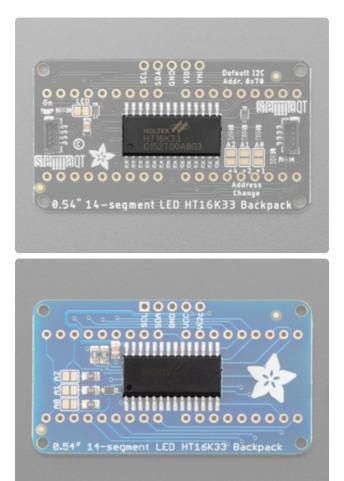
The chip located in the center of the back of the backpack is the HT16K33 matrix driver, which drives the 14-segment LED displays.
