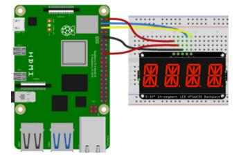
Pi GND to backpack GND (black wire) Pi 3.3V to backpack VIO (lower red wire) Pi SDA to backpack SDA (blue wire) Pi SCL to backpack SCL (yellow wire) Pi 5V to backpack VHi (upper red wire)
