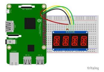
Raspberry Pi 3.3V to AlphaNumeric Display I2C VIN Raspberry Pi 3.3V to AlphaNumeric Display VIN Raspberry Pi GND to AlphaNumeric Display GND Raspberry Pi SCL to AlphaNumeric Display SCL Raspberry Pi SDA to AlphaNumeric Display SDA
