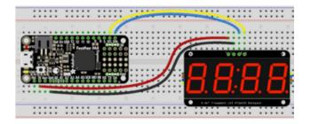
Microcontroller 3V to 7-Segment Display VIN (red wire) Microcontroller GND to 7-Segment Display GND (black wire) Microcontroller SCL to 7-Segment Display SCL (yellow wire) Microcontroller SDA to 7-Segment Display SDA (blue wire)
