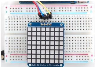
Place the soldered backpack on top of the header.
