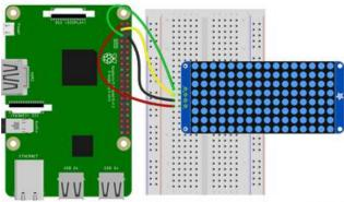
Raspberry Pi 3.3V to LED Matrix VIN Raspberry Pi GND to LED Matrix GND Raspberry Pi SCL to LED Matrix SCL Raspberry Pi SDA to LED Matrix SDA
