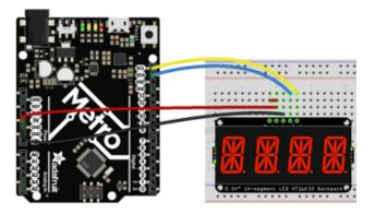
Board 5V to backpack Vio (long red wire) Board GND to backpack GND (black wire) Board SCL to backpack SCL (yellow wire) Board SDA to backpack SDA (blue wire) Backpack VIO to backpack VHi (short red wire)
