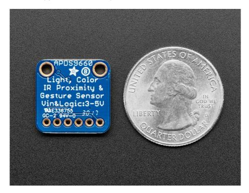
Since there are four IR sensors, you can measure the changes in light reflectance at each of the cardinal locations over time and turn those changes into gestures. Our interface library can detect directional gestures (left to right, right to
