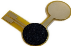
SEN0028 with NANOCOMP-CRC-10X10 material
