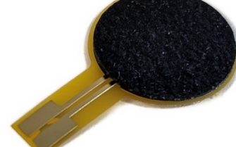
SEN0023 with NANOCOMP-CRC-15X15 material
