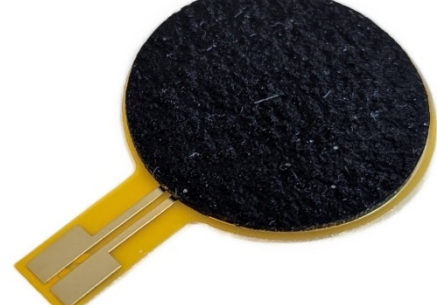
SEN0024 with NANOCOMP-CRC-20X20 material
