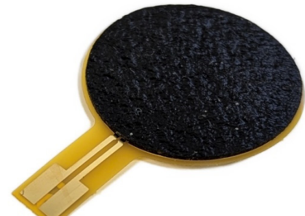
SEN0018 with NANOCOMP-CRC-20X20 material
