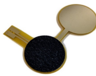
SEN0029 with NANOCOMP-CRC-15X15 material
