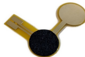
SEN0028 with NANOCOMP-CRC-10X10 material
