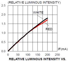
RELATIVE LUMINOUS INTENSITY VS. FORWARD CURRENT.
