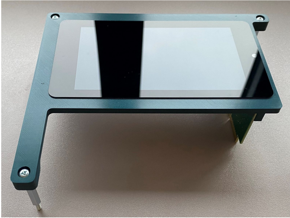
Fig. 1.8: Screwing standoffs to the jig
