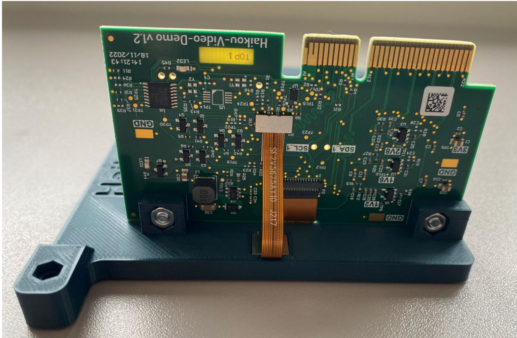
Fig. 1.6: Connecting camera to the Haikou Video Demo PCB
