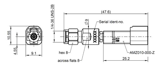
All dimensions are in mm; tolerances according to ISO 2768 m-H
