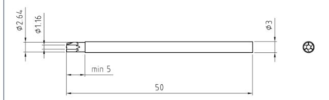
All dimensions are in mm; tolerances according to ISO 2768 m-H
