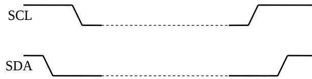
Figure 13. I 2 C Start and Stop Conditions
