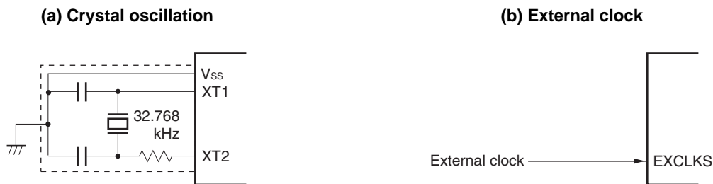
Figure 5-24. Example of External Circuit of XT1 Oscillator
