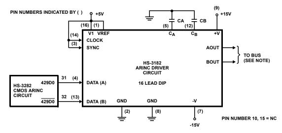
NOTE: The rise and fall time of the outputs are set to ARINC specified values by  $C_A$  and  $C_B$ . Typical  $C_A = C_B = 75$ pF for high speed and 300pF for low speed operation. The output HI and low levels are set to ARINC specifications by  $V_{REF}$ .
