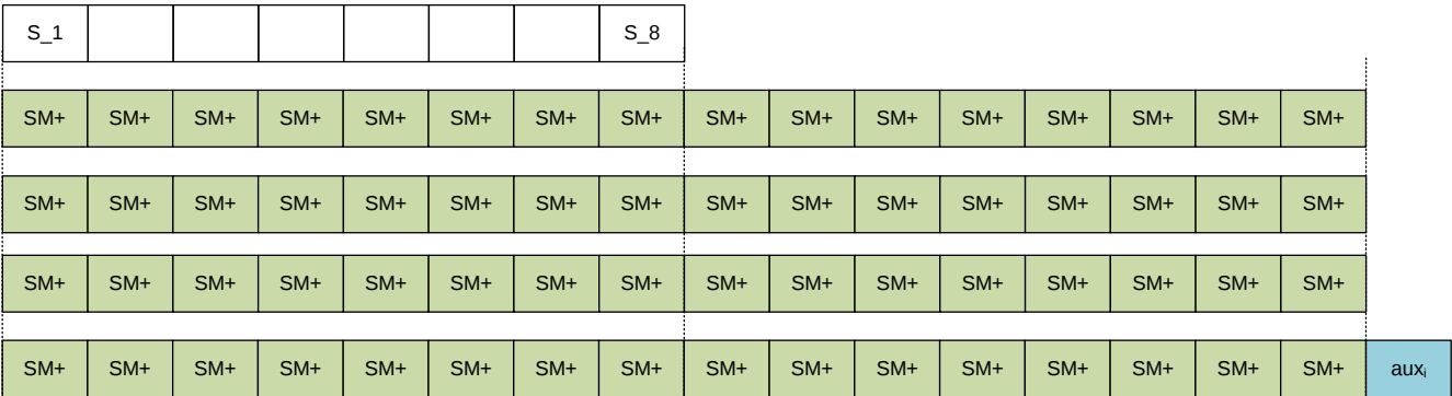
Figure 25: Sequencer Setup for Highest Update Rate on Bridge Sensor
