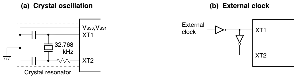
Figure 5-6. External Circuit of Subsystem Clock Oscillator
