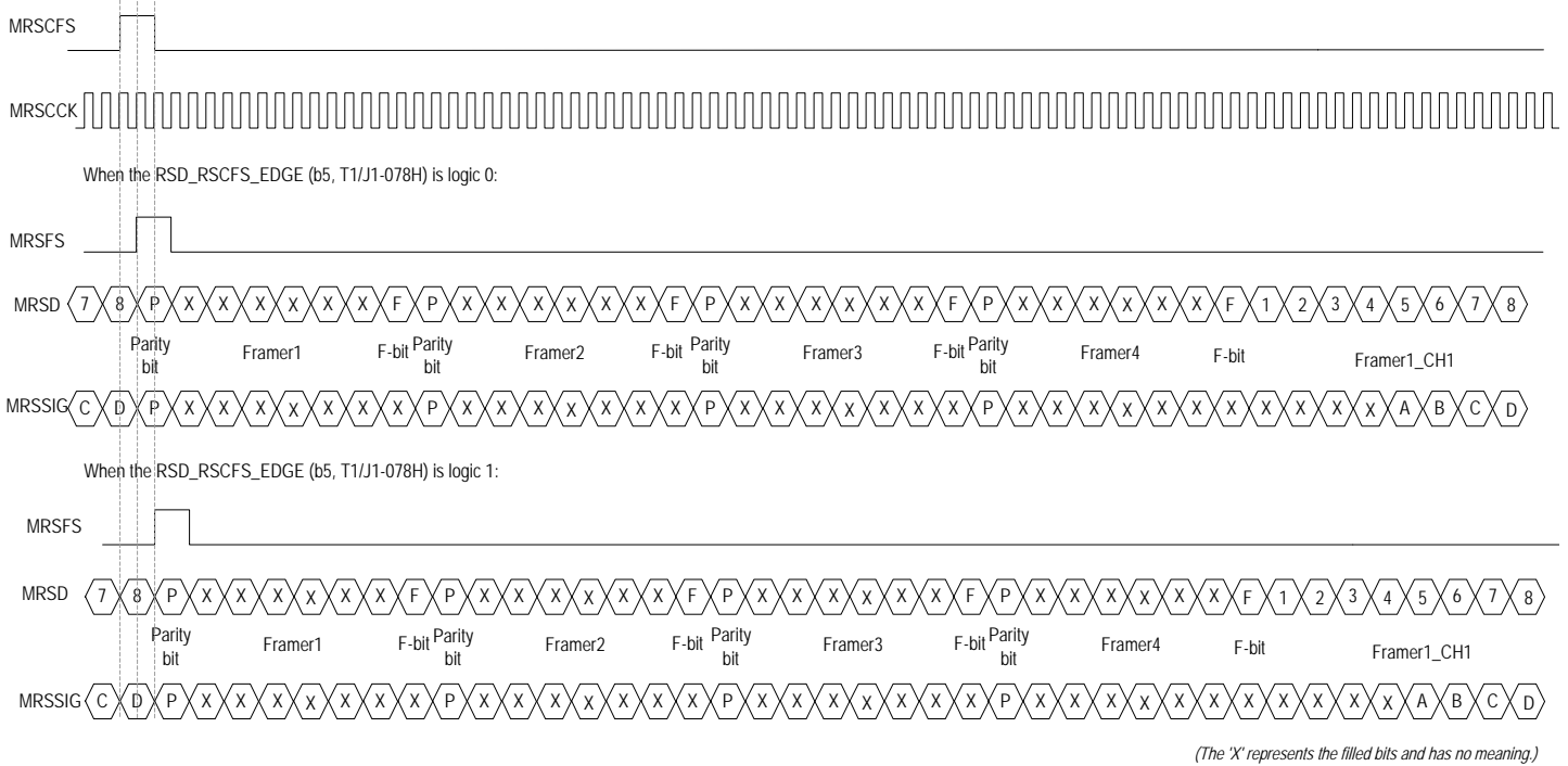
Figure 34. T1/J1 Receive Multiplexed Mode - Functional Timing Example 2
