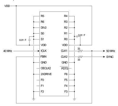
Note: The series termination resistor is located before the feedback trace.
