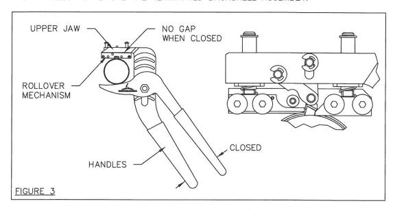
WARNING: DO NOT USE EXCESSIVE PRESSURE WHEN CLOSING THE ROLLOVER TOOL ON THE BAND. THIS MAY CAUSE DEFORMATION OR CRACKING.
