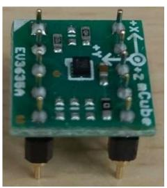
**R4, R5**: If using I2C and I2C pull-up resistors are needed for your application then install~4.7K $\Omega$  resistors into R4 (SCL clock pin) and R5 (SDA data pin) which are not installed by factory default. In addition, besides soldering resisters on R4/R5, you can add axial lead 4.7K ohm resistors to the SDA and SCL pin respectively. It will work the same either way.
