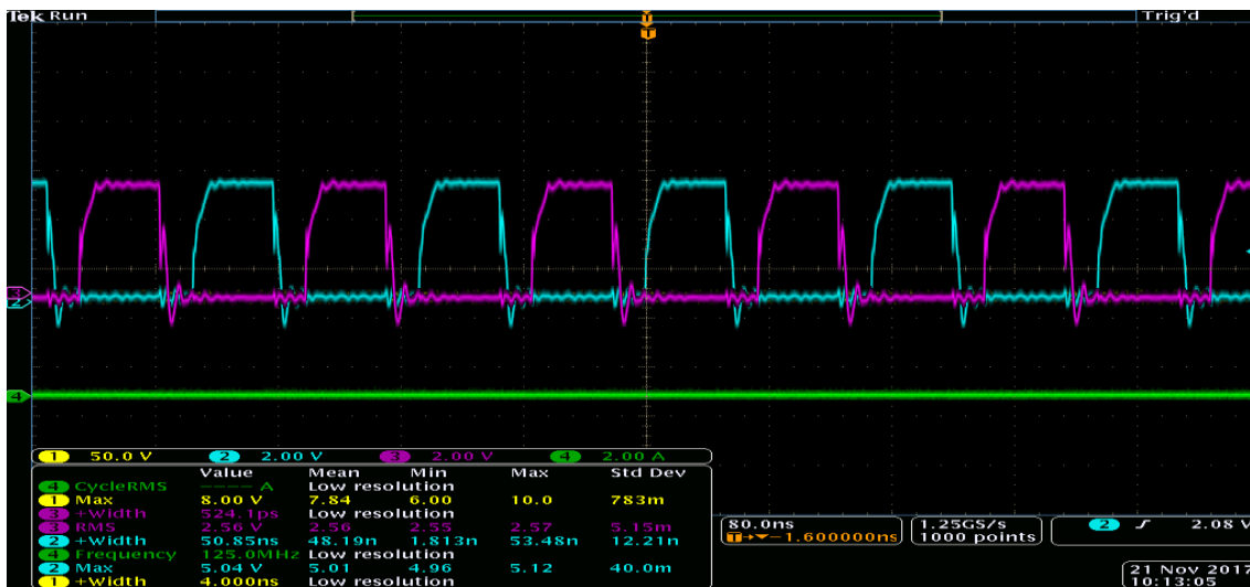
Figure 16 • Oscilloscope Plot Showing Both GS66508B Gate Node Signals at TP8, TP81
