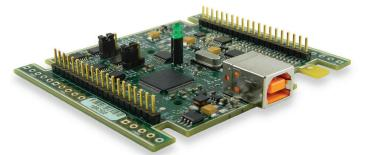
The USB-1208FS-Plus-OEM and USB-1408FS-Plus-OEM have the same specifications as the USB-1208FS-Plus/1408FS-Plus, but in a board-only form factor with header connectors instead of screw terminals.
