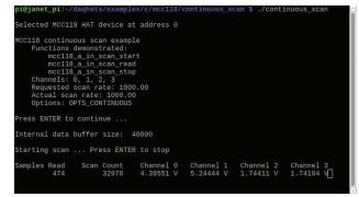
Display the value of each input channel in a terminal window
