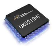
The Oxford Semiconductor OXU210HP is a single-chip, high-speed USB host and high-speed USB peripheral controller with integrated transceivers. It is the fourth controller in the family of integrated, low-cost, high-performance, On-The-Go (OTG) controllers that have been specifically designed for embedded systems.
