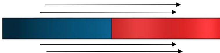
Figure 4: Multi-pole: Axial Magnetization
