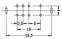
Recommended PCB Layout Top View
