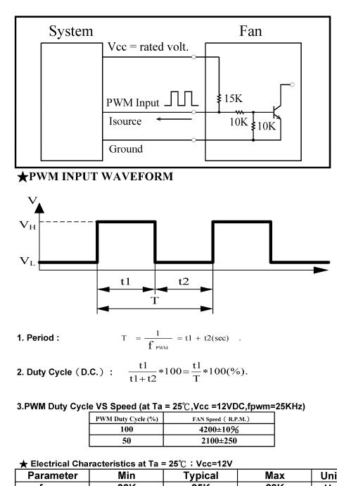
Unit f pwm 22K 25K 28K Ηz V<sub>H</sub> 2.3 5.5 V  $V_{L}$ 0 V \_ 0.8 Isource 0.8 mΑ 0 100 D.C. %
