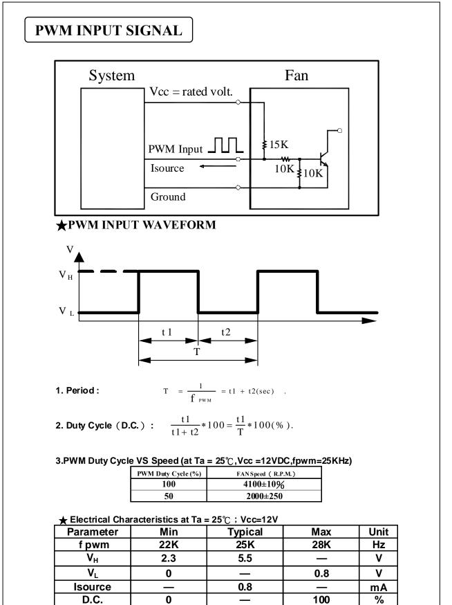
\* The speed is default to be maximum if PWM input pin is unconnected.
