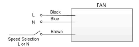
When the Black or Blue wire connect to Brown line, the Fan speed will switch to low speed mode.
