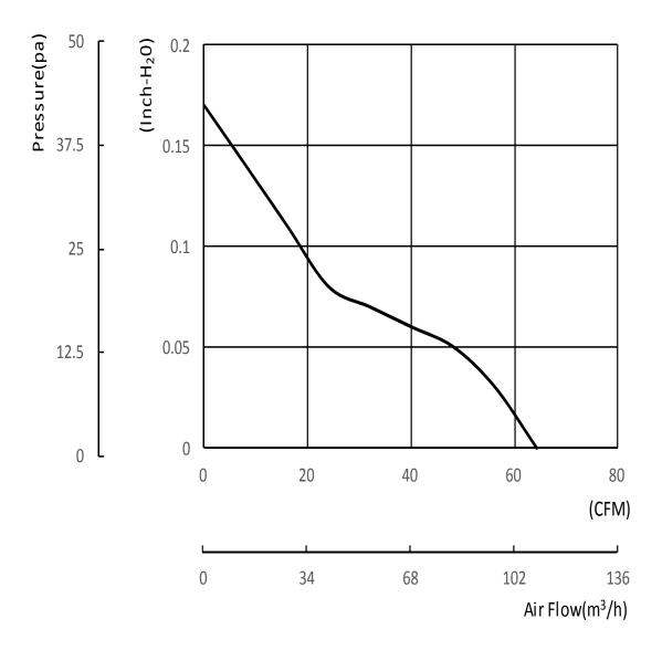
NOTE: The airflow and static pressure are measured with SUNON's specific fixture.
