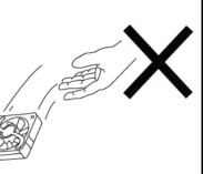
Don't cut the fan or lead wires
