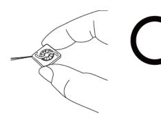
Don't pull fan with lead wires.
