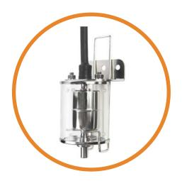
The SSF50 series is a compact vertical float switch with an integral acrylic slosh guard to reduce inadvertent operation in turbulent fluids. The unit can be mounted to a vertical surface or via a U-bolt (not supplied) using the integrated mounting bracket.
