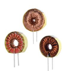
HTTI Series of High Current High Temperature Toroidal Inductors are vertical PCB THT mounted magnetics with a broad inductance and current range. HTTI parts employ a specific low core loss material with good DC saturation characteristics that is not subject to thermal aging making them suitable for operation at high temperature.
