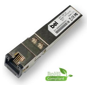
The Bel SFP-1GBT-09 transceiver is an internally configured 1000Base-T SFP module with Synchronous Ethernet capability for GBIC host interface. The host interface transmits and receives serial data differentially at 1.25Gbps. The copper interface is advertised as full duplex and 1000Base-T wire speed.
