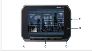
A. B. Speaker C. User-defined hotkeys D. Light sensor E. Reset, power, USB host (side)
