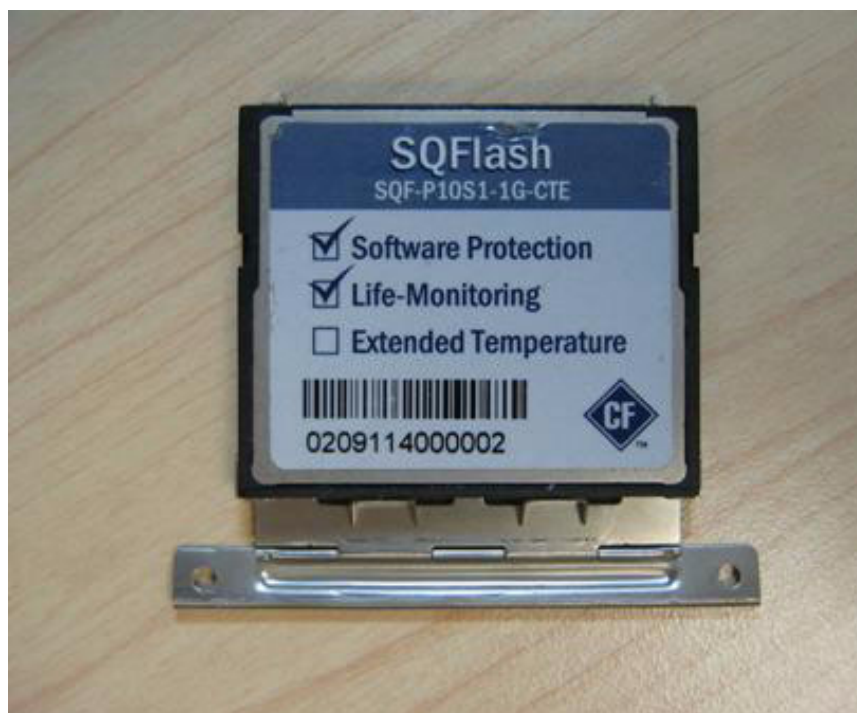
Figure 2.24 Put CF onto the CF tray
