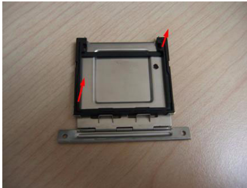
Figure 2.23 Remove CF bracket
