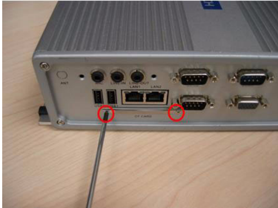
Figure 2.21 Unscrew the CF door screws
