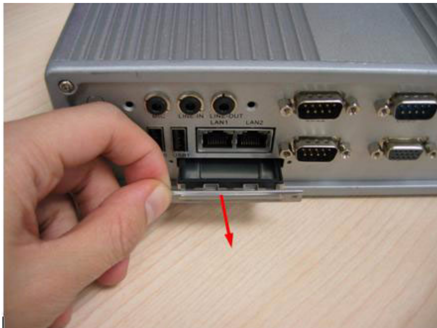
Figure 2.22 Pull the CF tray out
