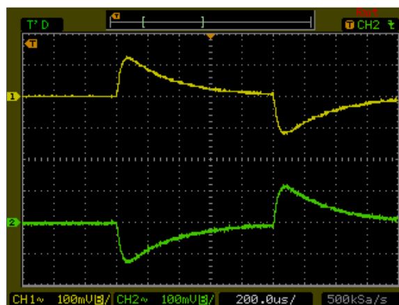
Figure 64: AXA000BB18-L Transient Response Vin = 24Vdc Load: Io = 100% to 75% load change Ch 1: Vo1 Ch2: Vo2
