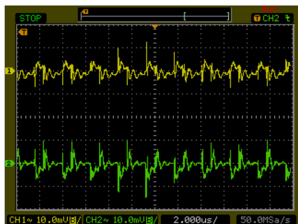
Figure 73: AXA000CC18-L Ripple and Noise Measurement Vin = 24Vdc Load: Io = \pm 0.33 A Ch 1: Vo1 Ch2: Vo2
