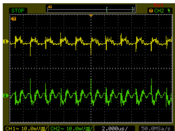
Figure 63: AXA000BB18-L Ripple and Noise Measurement Vin = 24Vdc Load: Io = \pm 0.41 A Ch 1: Vo1 Ch2: Vo2
