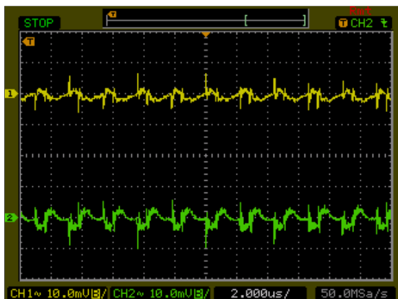
Figure 53: AXA00AA18-L Ripple and Noise Measurement Vin = 24Vdc Load: Io = \pm 1 A Ch 1: Vo1 Ch2: Vo2
