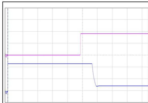
Figure 6: AVO120-48S12 Output Shutdown by Remote Off (100ms/div)
