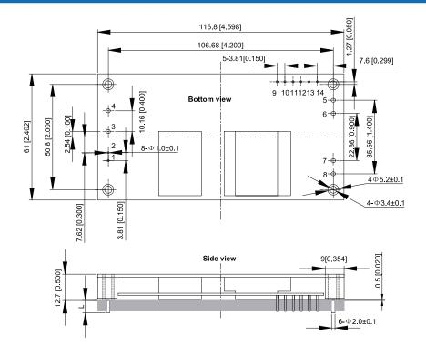
Unit: mm[inch] Bottom view: pin on upside Tolerance: X.Xmm±0.5mm[X.X in.±0.02in.] X.XXmm±0.25mm[X.XX in.±0.01in.]
