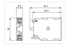
B = Spring-type terminal for Part No. 45-315.1Z40, 45-315.1X40
