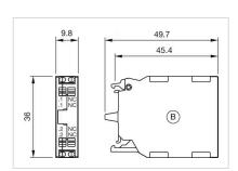
B = Spring-type terminal for Part No. 45-314.1Z40, 45-314.1X40
