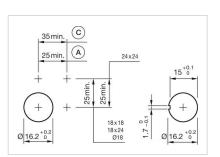
$\begin{array}{l} A = Solder/Plug-in \ terminal \ 2.8 \ mm \ x \ 0.5 \\ mm \\ C = Screw \ terminal \end{array}$
