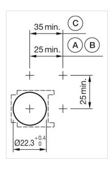
A = Solder/Plug-in terminal 2.8 mm x 0.5
